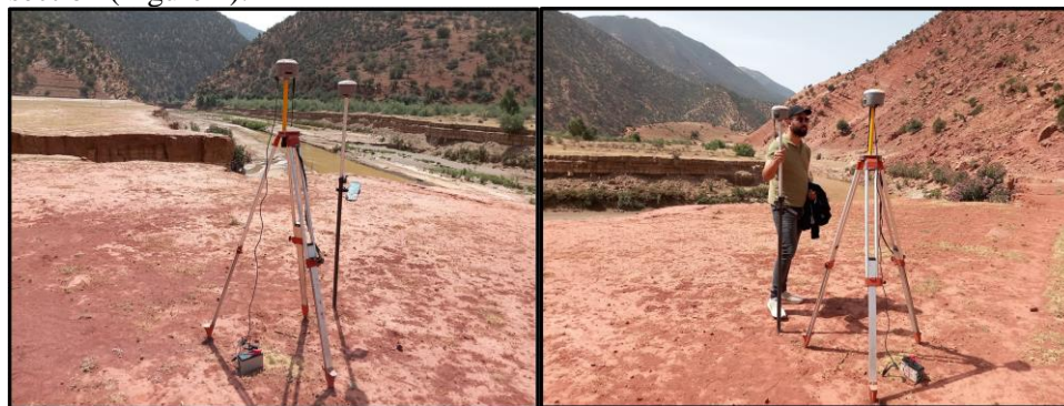
Figure 2. Total topographic station used for extracting topographic sections
